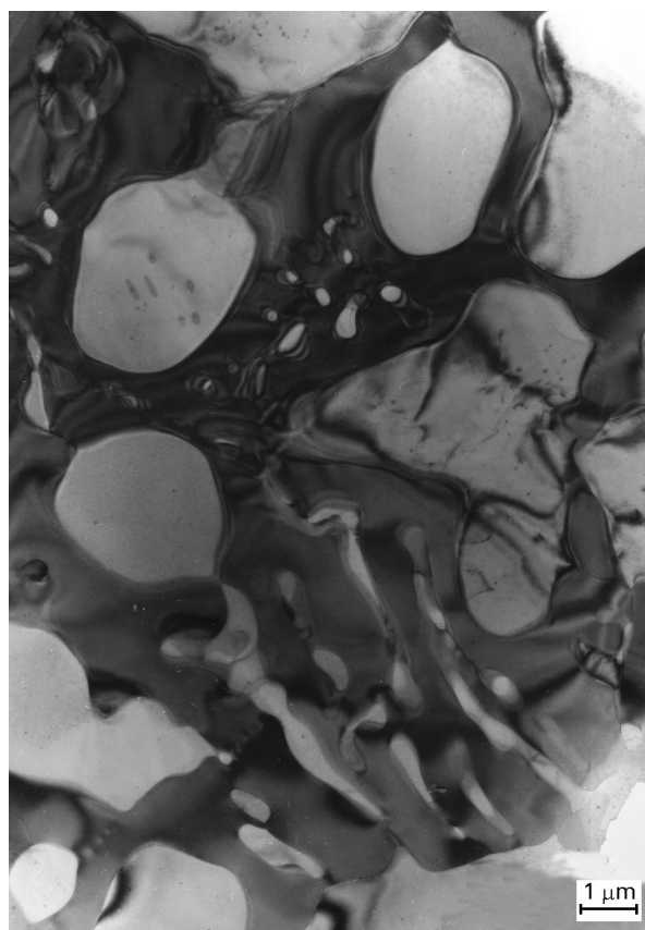
Figure 5 Bright field electron micrograph of a typical region in the AlGe45 as-quenched ribbon.
